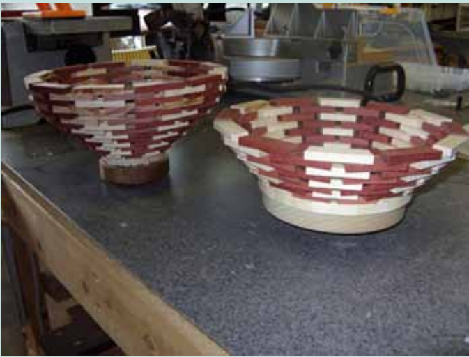
13. The two pieces of the form all glued up and ready to be turned.
