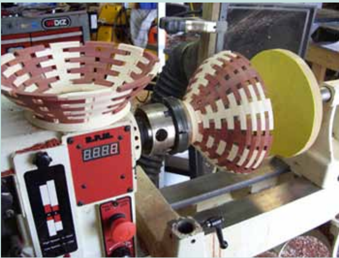
15. This is the fun but scary part. Turn both pieces smooth inside and out. Be sure the diameter and wall thickness is the same on both parts. I use a disk with stick-on foam to secure the piece while I turn the outside. When both parts are turned it is time to glue them together on the lathe. Once they are dry, part off the block at the top and smooth the inside joint. Bring up the tailstock with stabilizer disk and clean up the outside joint. Sand to desired finish then part off the bottom.
