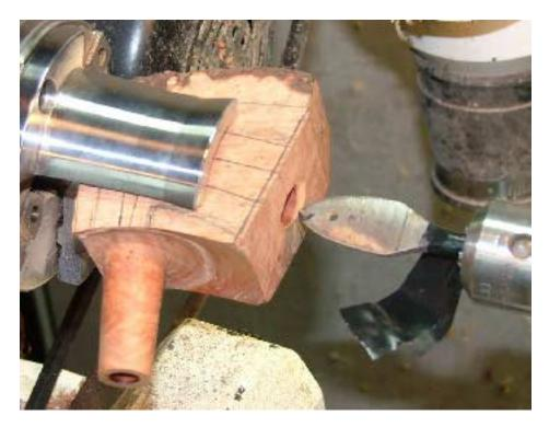
As you can see, the tobacco chamber stops just as it hits the bottom of the smoke hole.
