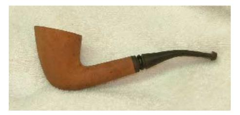
Then I hand sand to 220 grit and apply a second coat of dye. This process is repeated with 320 and then 400 grit. After sanding with 400 grit I apply the last coat of dye which does not get sanded back.
