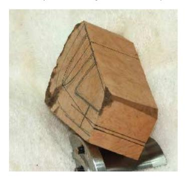
Place the block in a 4 jaw chuck with two of the jaws removed.
