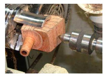
As with the other drilling I used the tip of a skew chisel to make an entrance hole. Drill out the tobacco chamber only part way with a large diameter drill bit. I am using  $\frac{1}{2}$ " here.
