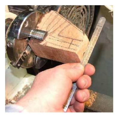
When drilling the hole for the stem you need to stop frequently and check your progress. When making a bent pipe it is critical that you stop drilling the stem hole when the smoke hole is centered in the stem mortise hole. (Remember that the smoke hole and the stem hole are not parallel in a bent pipe.)
