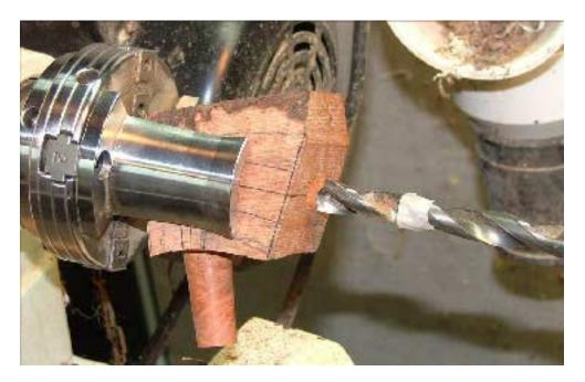
Now you can take a spade bit, which has been ground to the desired shape and sharpened like a scrapper, to drill your tobacco chamber.
