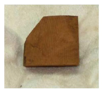
Once the sides are squared up you can draw your design on one face of the briar. Note that you need an accurate line for the center of the bowl, the smoke hole and the stem hole. On a straight pipe the smoke and stem holes are on the same line.
