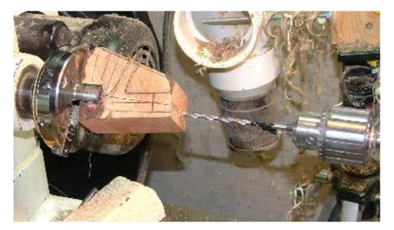
Re-chuck and re-center the block along the guide line for the stem. Again, make a starting hole for the drill with the tip of a skew chisel. When drilling the hole for the stem go slow and clear shavings every <sup>1</sup>/<sub>4</sub> inch or less. I used a 5/16" bit for the stem tenon.
