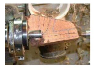
Put a Jacobs chuck into the tailstock and drill the smoke hole.
