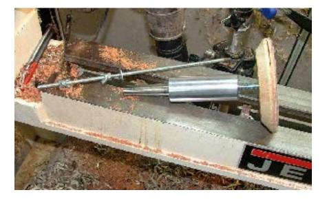
And I am ready to rough sand. Ventilation is a must here. Watch your knuckles and also the parts of the pipe you don't want to sand.
