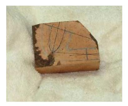
Transfer your three lines onto the top and side of the block. (You must be very accurate here since you will be using these lines to drill your holes.
