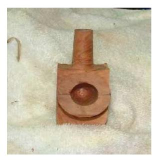
Then you can clean up the chamber with a small scrapper or some sand paper wrapped around a dowel rod.
