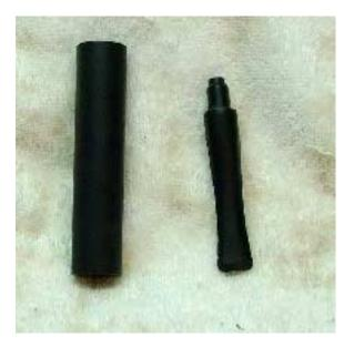
Find a drill bit that will just fit in the draft hole in the stem.
