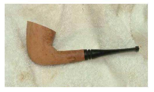
Here I have completed final shaping and have hand sanded the pipe to 150 grit.
